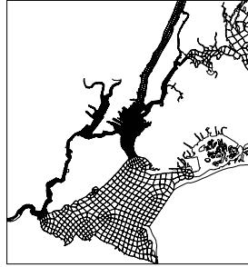
Fig. 3. Spectral element grid showing elemental partition of the New York/Newark Bay estuarine system
